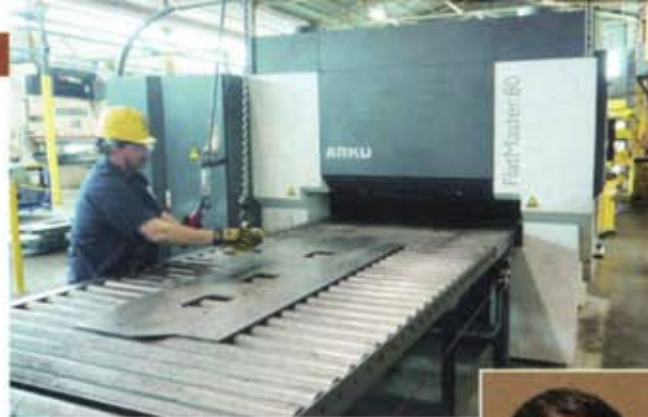
A free-standing servo-hydraulic leveler integrates easily into fab shop workflow to supply stress-free parts for bending, assembly or welding.
